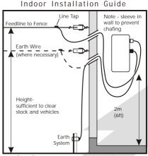
driven 6.5 ft (2 m) into the soil and spaced at least 10 ft (3 m) apart. A minimum of two earth rods is recommended.
